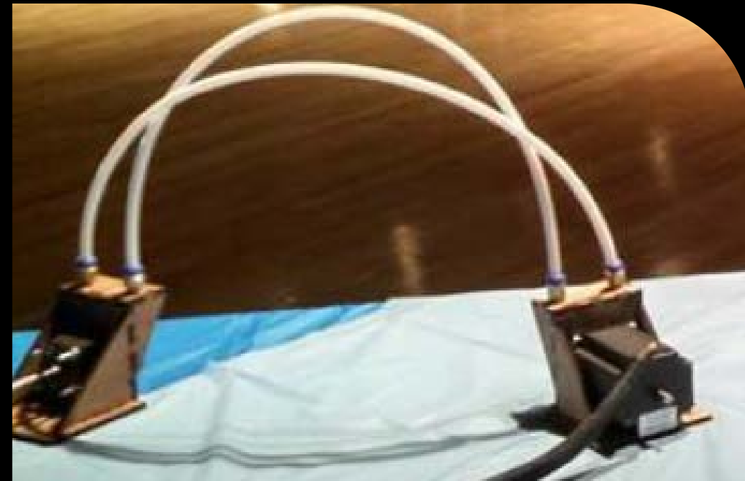
Bead chain routed from motor (right), through PTFE Bowden tubing, to an output shaft (left).
